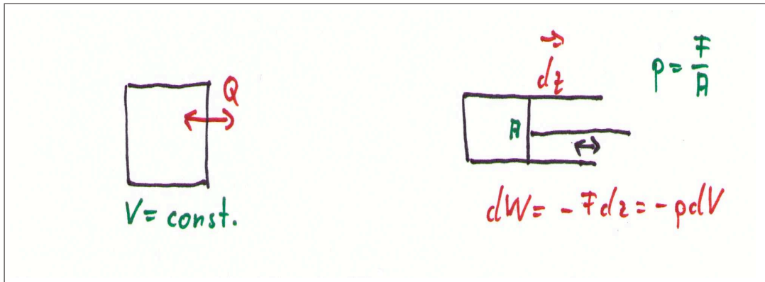
FIG. 37: Exchange of heat and work with the environment
